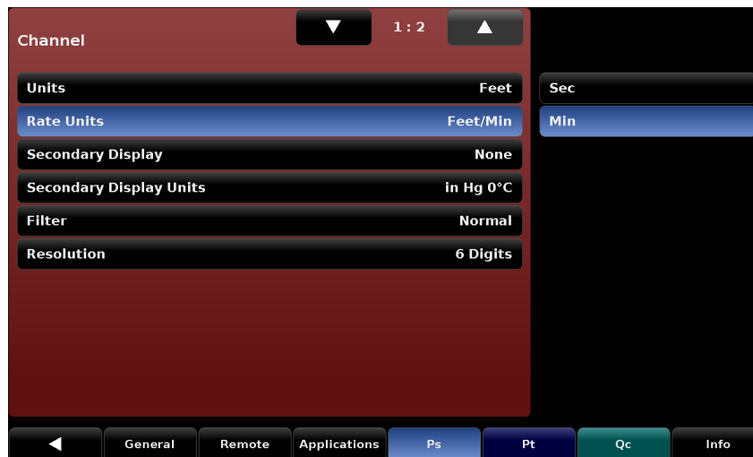
Figure 7.3.2 - Ps Rate Units (showing Feet/Min)
