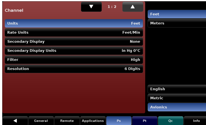
Figure 7.3.1 - Ps units menu showing English units
