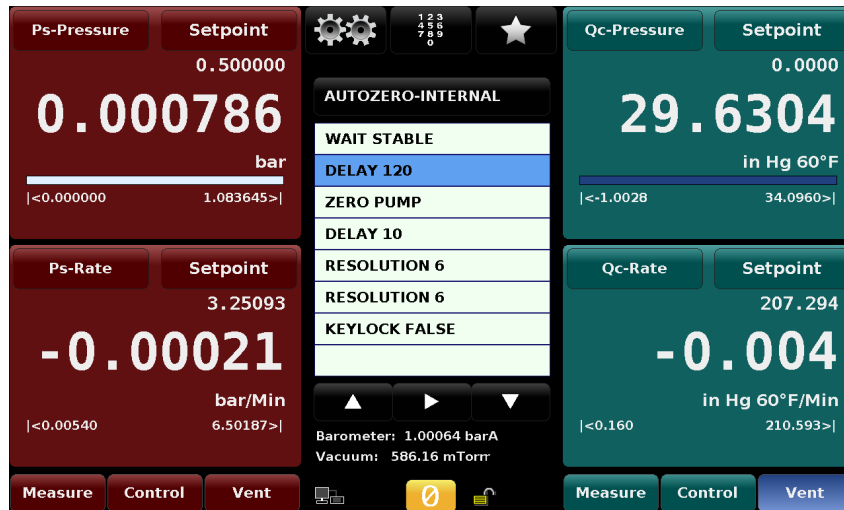
Figure 6.2.14c - Zero Sequence, 120 second delay
