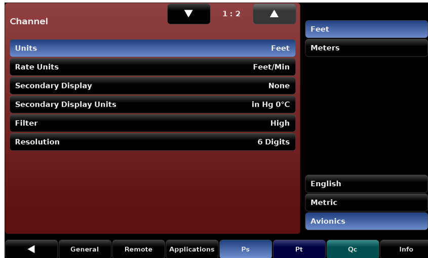
Figure 7.3a - Channel Page of Ps Setup
