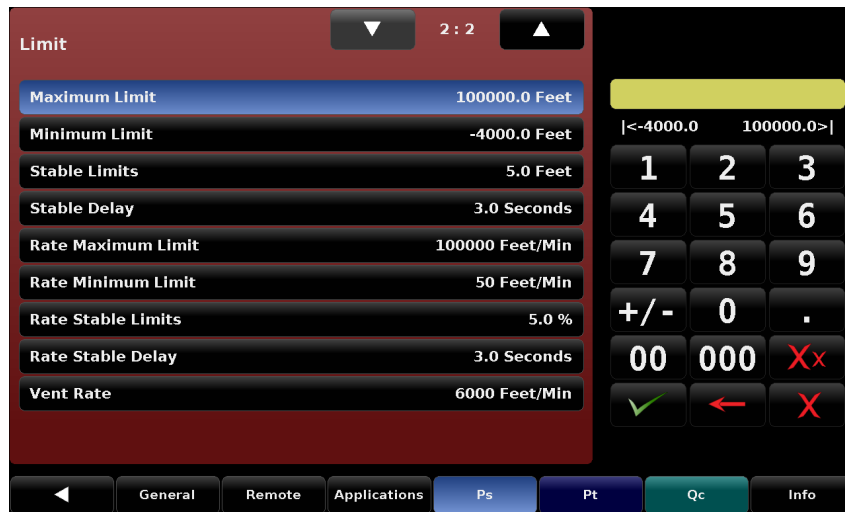
Figure 7.3b - Limit Page of Ps Setup
