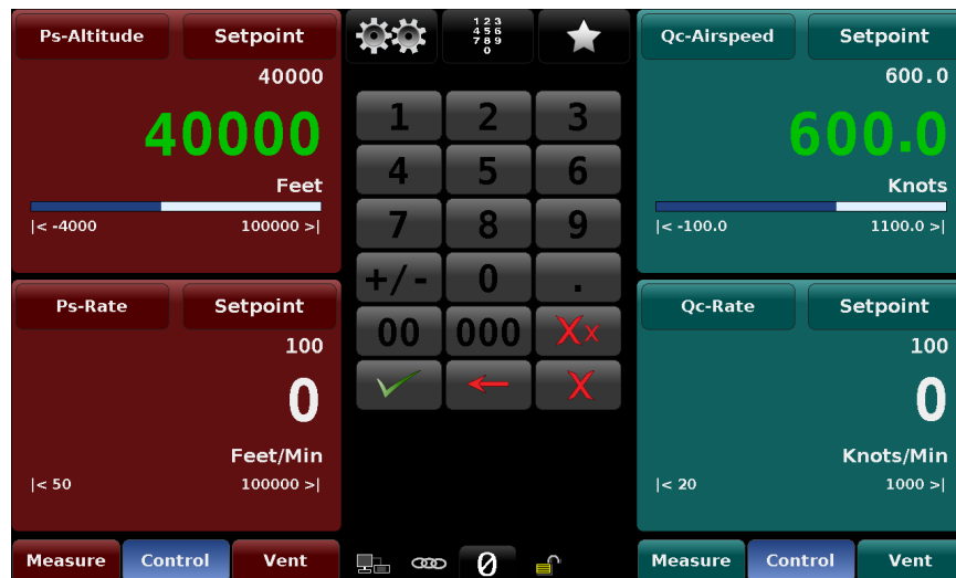
Figure 6.2.2 - Altitude and Airspeed Reading (shown in green)
