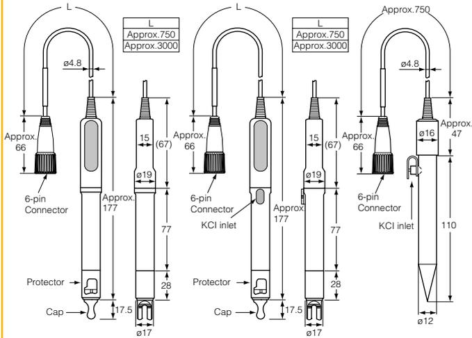
Test tube size pH sensor
